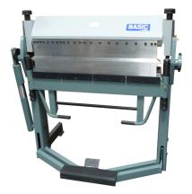
The segment folding machine is used to fold metal, create leader heads and liner trays
